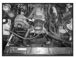
Step 13 Install the coupler on the throttle body and secure the coupler in place. Install a second clamp but do not tighten at this time.
