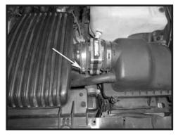
Step 4 Loosen the clamp on the outlet side of the Mass Air Flow Sensor (MAFS). Remove the air intake tube assembly including the factory tube coupler from the vehicle.
