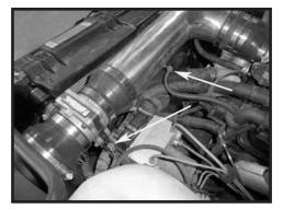
Step 16 Reconnect the MAFS electrical connector and install the small vent hose into the grommet.
