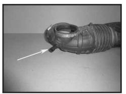
Step 10 Remove the IAT sensor from the factory intake tube.
