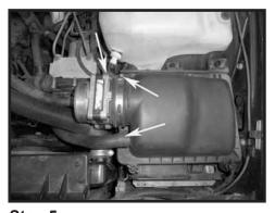
Step 5 Disconnect the PCV fresh air hose from the air box and electrical connector at the MAFS. Loosen the clamp for the inlet side of the MAFS and remove the MAFS from the vehicle.
