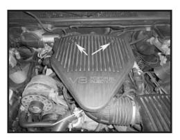
Step 2 Remove the two nuts and loosen the clamp. Remove the engine cover from the vehicle.
