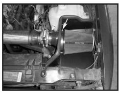
Step 17 Install the supplied air filter and clamp and tighten the clamp that secures the air filter. If needed, rotate the air filter/velocity stack adapter assembly for the maximum clearance as shown.
