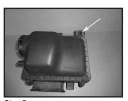
Step 7 Remove the factory grommet from the air box. This will be reused in Step 8.
