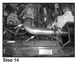
Install the factory PCV hose to the fitting on the bottom side of the intake tube. Install the Spectre Performance intake tube into the coupler on the heat shield then into the coupler on the throttle body. Fasten securely in place.
